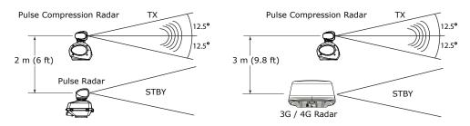
**Do not** install the Halo® pulse compression radar on the same beam plane as a conventional pulse radar. A pulse radar must be set to STBY or OFF any time the Halo® radar is being operated.
