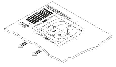
Drill pilot holes, Then use a 12.5 mm (1/2") drill bit to drill the four holes where shown on the mounting template.
