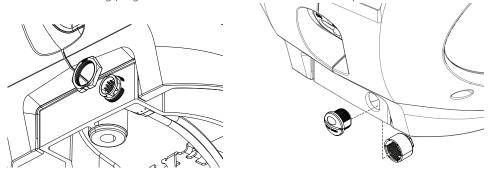
3. Re-route the internal fly lead to the bracket and secure with the nut.
