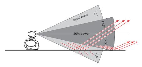
For best performance, the radar should be positioned to allow the beams to clear the superstructure of the boat.
