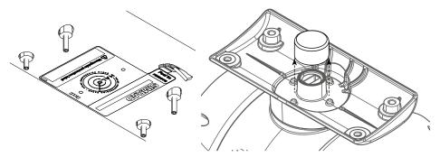
2. Carefully lower the antenna on to the pedestal. The antenna can only fit one way
