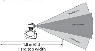
Below is a guide to determine the antenna height in relation to a vessels hard top overall width. Every Increase of 200 mm (7.9") of hard top total width over 1.8m wide: Increase the height of the antenna by 46 mm (1.8")
